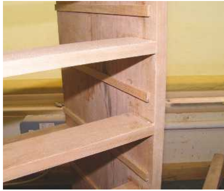
▲ Pic.20 The drawer runners were thin strips of cherry glued and pinned to the side panels
